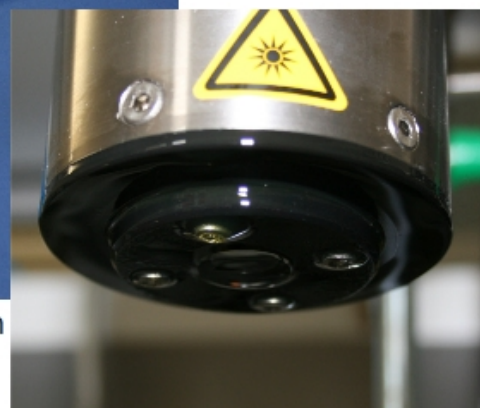
A new innovative nano-coating on the optical lens prevents oil-films and fouling
